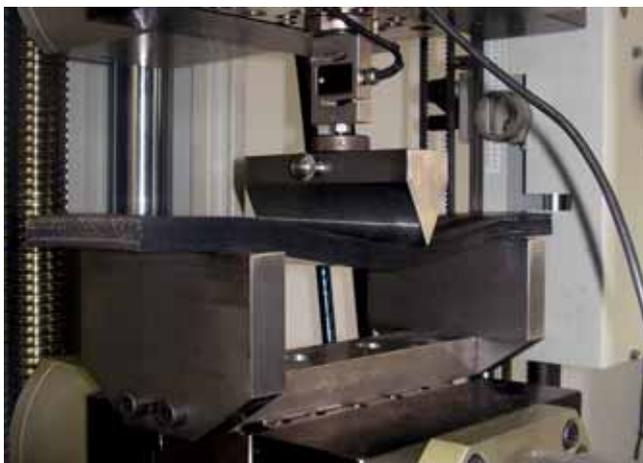
*Fig. 4: Sealtex transversal bending test clearly shows how abnormal and not linear the deformation of the sample is, with respect to the behaviour of a simple steel beam.*
